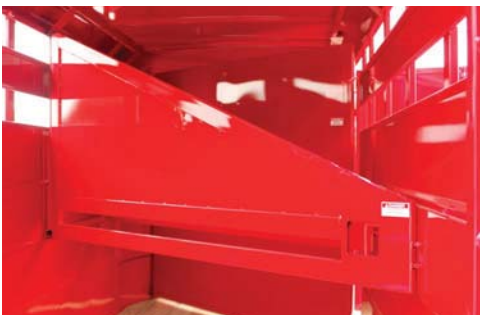
New Slant Divider Latching Mechanism
