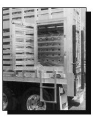
Driver's side rear access door includes convenient fold-down step.
