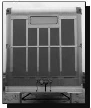
Fully ventilated front end shown with optional panels installed (lighted sign is optional).
