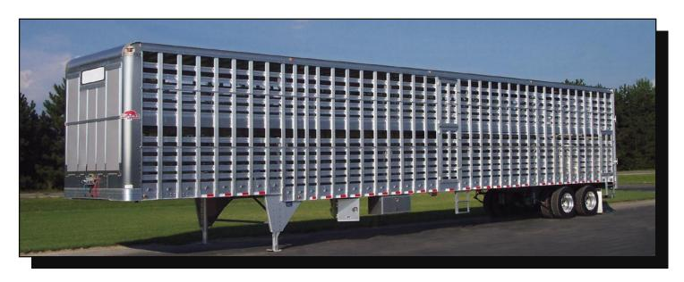
Featured: Drop Deck Slat Side, available in lengths to 53". Shown with popular Eby Trans Pork options: fully vented front-end with closure panels. Slide-in side winter closure panels with storage and other options not considered standard.
