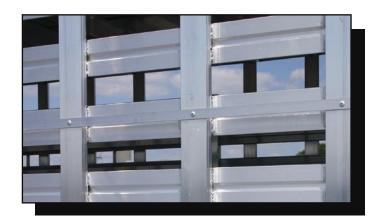
Superior ventilation- proven post and slat design provides maximum air flow with the most air openings in the industry! Size and location of openings can be placed as determined by your air and cargo requirements. All models feature slotted closure posts for future winter panel use.
