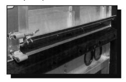
Rear wash-out panel provides better curbside drainage; hinges down to prevent runout when trailer is in use.
