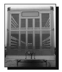
Fully ventilated front end shown with panels removed (lighted sign is optional).
